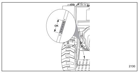
Figure 3-1 Engine Oil Level Check
